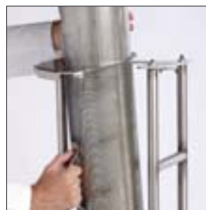
The strainer cylinder and screw conveyor are easily accessible and removable.
