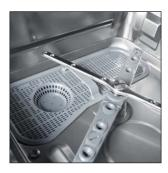
The wide angle nozzles FAN spray the water with greater accuracy in a much wider range...
